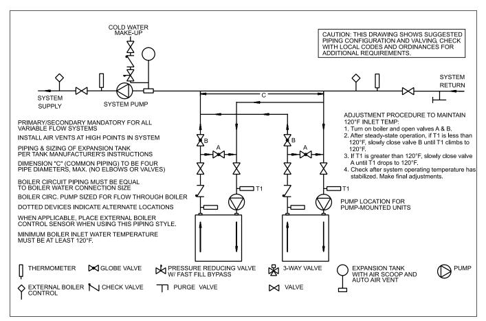
Figure 8. Hydronic Piping — Primary-Secondary, Reverse-Return, Low Temperature.
